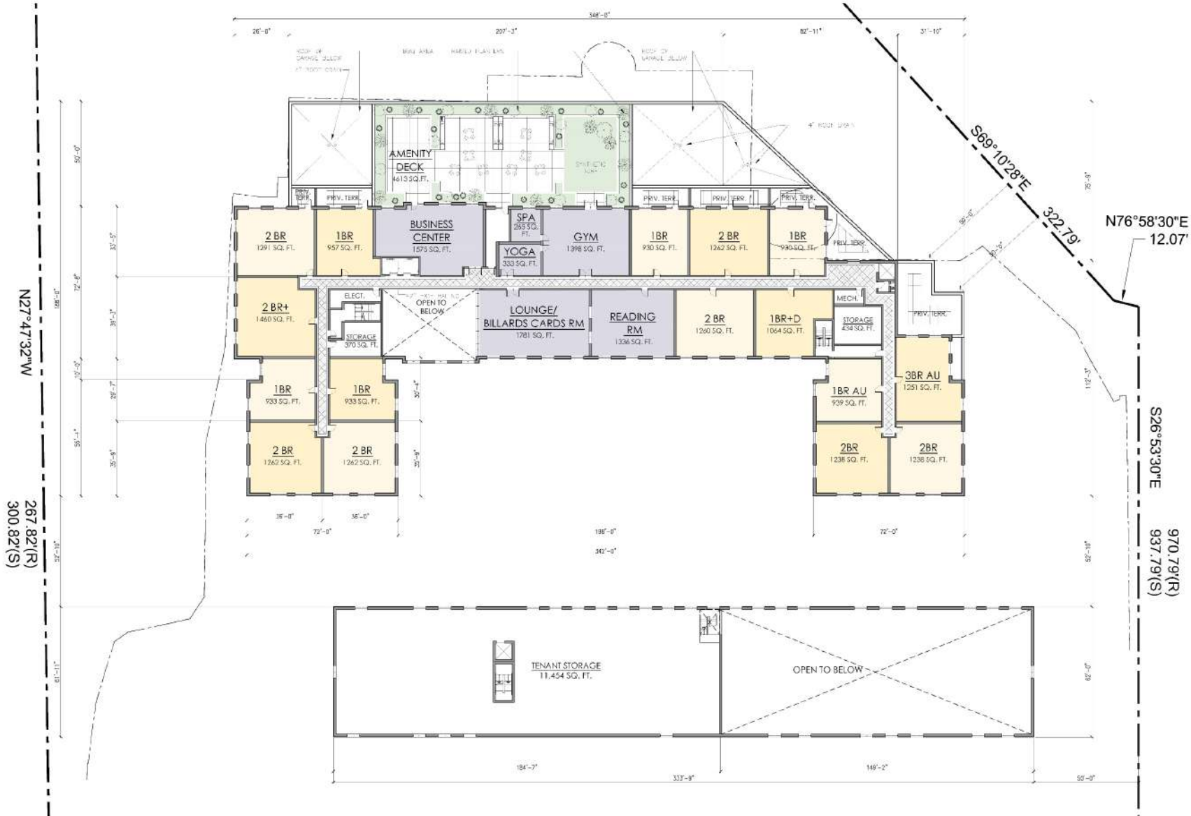
1 SECOND FLOOR PLAN SCALE: 1/20"=1'-0" 0' 4' 8' 16'
