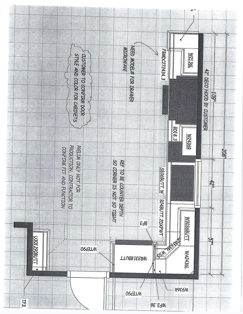
208" . 13" 21" 48" 24" 48" 30" 24" 109" 42" 57" ັດ. 33" HOOD-42 W2139L 59" 48" 53" W3039BUTT WA2439L Ö 196 TPP122493L ٠. . . <del>-</del>:: 54" 36" FBMDC272434\_1 ANGE.GAS.36-2 BD18.3 DISHW18 SB36BUTT.W IBUTT.2DXFWTZR3633L.WSS 1" 12" · 27" 36" 18" 36" 36" 58" 45" 27" 78"
